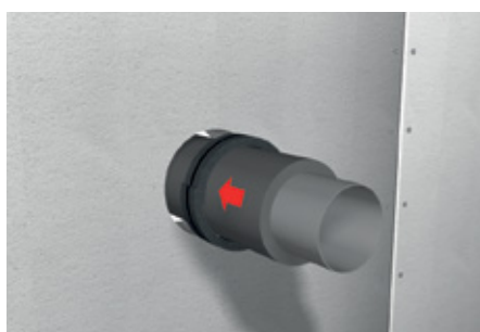
7. PROMASTOP®-W shall be installed flush with the penetration seal or wall surface, maximum 5 mm in front of the wall/floor
